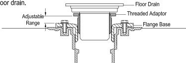
3. If using a rubber adaptor, make sure the rubber adaptor is fully pushed in the flange base. Gently pull up or press down the floor drain to adjust the installation height of the floor drain.
