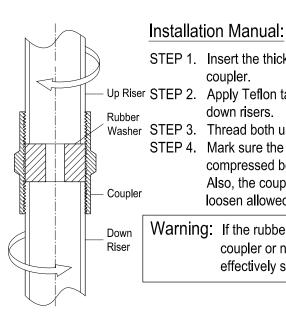
STEP 1. Insert the thick rubber washer inside the
