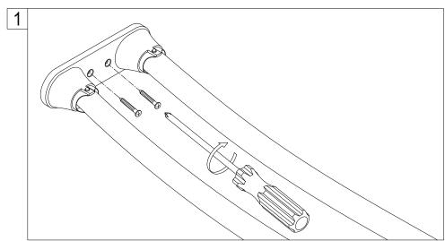
1. Locate where you would like to install the curved shower rod. Place a base onto the wall and trace around it with a pencil.
