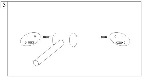
3. Insert anchors into the holes with a hammer until flush with the wall.
