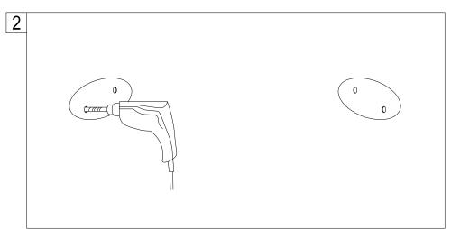
2. Place the mounting plate in the center of the pencil outline you just made and mark the location of the mounting screws.
