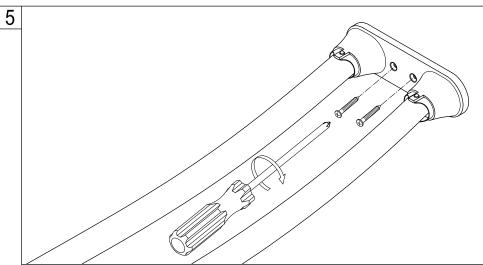
5. Expand the shower rod and install on opposite end. Repeat steps 1 through 4 with the other side.
