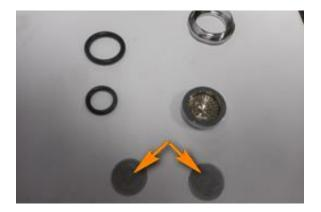
4. Clean thoroughly. This should remove all debris that may be in the spray head or in the aerator.
