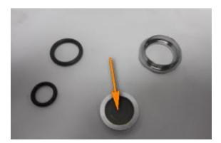
3. Remove the washers and carefully remove the mesh.
