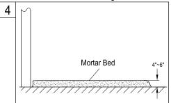
4. Pour a generous, (4" to 6") layer of mortar mix cement to the area where your tub basin will be sitting, please note that due to the tubs slope, it is necessary to apply a thicker layer on the side opposite the drain, make sure to cover the drain to prevent any mortar from falling inside, leave the area where the feet will be resting free of mortar as well.
