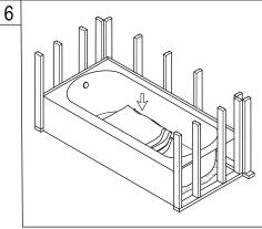
6. Secure to the wall with galvanized screws at the predrilled screw location, apply weight to the middle of the tub until the mortar sets.
