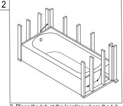
2. Place the tub at the location where the tub will be installed, level tub on all sides, deck should be level or have a slight slope towards the tub, it might be necessary to adjust the 1" x 4" lumber supports to insure proper deck drainage, mark the location of the drain and the wall studs on the tile flange.
