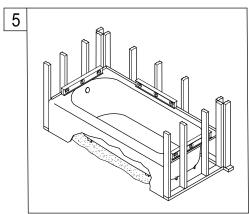
5. Set tub into place, make sure the tub is level, make sure that the mortar bed is in contact with the entire tub basin.
