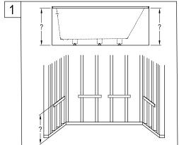
1. Prepare area by framing the area where the tub will be installed, measure the distance from the floor to the bottom of the tub lip, using that measurement attach a 1" x 4" piece of lumber on the walls where the tub will be secured.
