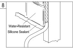
8. Install water resistant gypsum board and finish surface material (tile, stone) and seal all edges with silicone caulking to prevent water damage.
