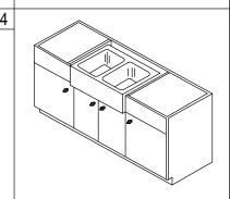
4. Install the sink in the opening, check that the sink is level from side to side and front to back, add wood shims if necessary, once sink has been leveled, fill the gaps using silicone caulking.
