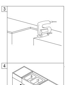
3. Cut the countertop along the template line and add 1/8" to the height of the sink and cut front of the cabinet using that dimension with the proper tool for the countertop material, sink should be supported by the 2" x 4" supports not the cabinet front, depending on the configuration of your base cabinet, it may be necessary to remove the doors and replace them with smaller doors.
