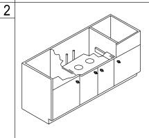
2. Install 2" x 4" supports across the base cabinet, the sink should be able to sit on top of the supports and its top rim should be at a point right below the finished countertop.
