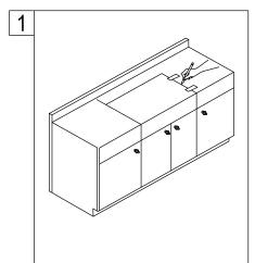
Cut out the template and place it on the countertop, making sure that the sink front is parallel to the front of the counter. Be sure the sink is properly centered, both front to back and side to side.
