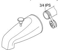
Step 2. Thread spout onto pipe.
