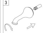
3. Slide the spout over the pipe. With the spout tight to the wall, tighten the set screw to the pipe.
