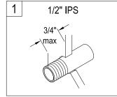
1. The stub-out pipe for spout installation must be at the length illustrated measured from the finished wall surface.
