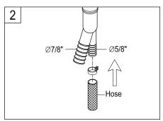
2. Attach 5/8" dishwasher drain hose to 5/8" leg. Secure with hose clamp.
