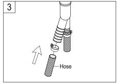
3. Attach 7/8" garbage disposal hose or side inlet sink trap drain hose to 7/8" leg. Secure with hose clamp.
