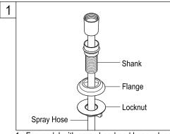
1. For model with spray head and hose, place the spray guide through the fourth hole in the sink, screw the locknut onto the shank and tighten firmly.
