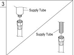
3. Connect spray hose to hose outlet located underneath the faucet.
