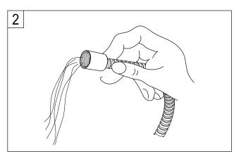
2. Open water to flush the sprayer hose before installing with sprayer head.
