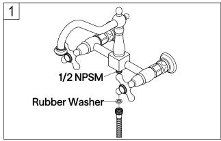
1. Place rubber washer and connect spray hose to hose outlet located underneath the faucet.
