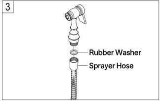
3. Place rubber washer to end of spray hose and attach sprayer.
