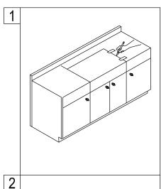
Cut out the template and place it on the countertop, making sure that the sink front is parallel to the front of the counter. Be sure the sink is properly centered, both front to back and side to side.
