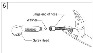
5. Place the bigger rubber washer inside the spray hose adapter. Install spray head by threading it clockwise onto the adapter. Tighten it by hand, but do not over-tighten, as this can cause damage and leaks.
