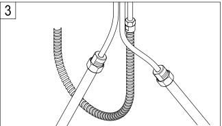
3. Connect the supply lines onto the cold and hot inlets.
