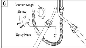
6. Install the counter weight on spray hose by tightening up the screws. Turn on water at least 1 minute to check for leaks. If any leak is found, loosen the connection, clean out debris, and reassemble the spray hose.
