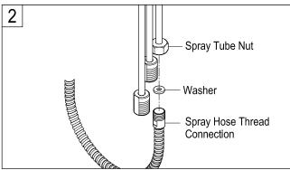
2. Place the smaller rubber washer inside the spray tube nut. Connect the spray hose thread with the spray tube nut by hand. Then gently tighten up the nut using an adjustable wrench. **Do Not Over-tighten**.
