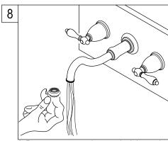
8. Remove aerator and turn on both hot and cold valve, let water run for at least 1 minute, this will clear any debris remaining on the waterways, replace aerator.
