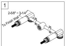
Properly secure valve body to wood bracing using copper straps, make sure to place body so that the distance between the back of the valve body to the finish wall surface is 2-5/8" to 3-1/4".
