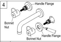
After applying silicone based caulking to the back of the handle flanges insert onto valve body and push completely to the wall, and thread bonnet nut onto valve assembly.
