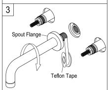
3. After inserting the spout flange, apply Teflon tape to spout and thread spout onto valve body. Turn the spout clockwise by hand to connect with valve body. Make sure it is tightly connected, then adjust slightly to ensure the spout outlet is facing down. Apply silicone based caulking to the back of the flange and press against the wall.
