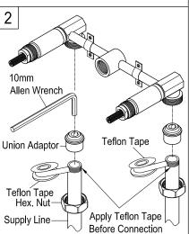
2. Connect valve assembly to 1/2" IPS supply lines, the union adaptors on this valve are threaded for 1/2" NPT male threaded fittings.
