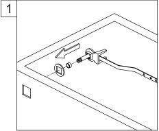
Insert plastic washer and flush arm through bracket, then place rubber washer onto bracket.
