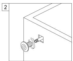
2. Slide lock nut assembly over end of flush arm from front and tighten by hand or adjustable wrench.
