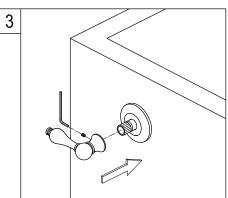
3. Position handle to the right or left depending on preference and secure by tightening set screw on the side of the handle or in certain applications it may have a screw in the center of the handle, after securing handle, placed decorative handle cap (certain models only) onto handle.
