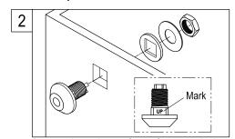
2. Insert the tank lever flange from outside the tank, make sure the word "UP" is visible from the top, insert rubber and metal washer and secure by threading locknut, be careful not to overtighten as this may damage the tank.
