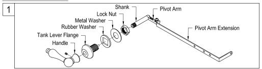
1.Remove the handle by unthreading the set screw holding the handle, and disassemble the tank lever assembly, remove the brass locknut, metal washer and rubber washer.
