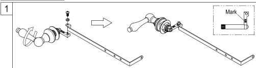
1. Remove pivot arm extension from the pivot arm by unscrewing the Phillip's head screw, flip pivot arm so that the word "Side" is visible from the top, reinstall pivot arm extension, making sure that the notch on the pivot arm extension fits on the pin on top of the pivot arm.
