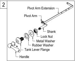
2. Remove the handle by unthreading the set screw holding the handle, and disassemble the tank lever assembly, remove the brass locknut, metal washer and rubber washer.
