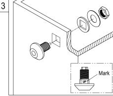
3. Insert the tank lever flange from outside the tank, make sure the word "UP" is visible from the top, insert rubber and metal washer and secure by threading locknut, be careful not to overtighten as this may damage the tank.
