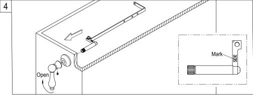
4. Insert tank lever shank into the tank lever flange assembly, insert lever on the protruding shank and secure by tightening set screw, make sure the word "SIDE" on the pivot arm is visible from the top, the pivot arm extension can be bent to fit your specific tank.
