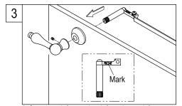
3. Insert tank lever shank into the tank lever flange assembly, insert lever on the protruding shank and secure by tightening set screw, make sure the word "FRONT" on the pivot arm is visible from the top, if it's not visible remove the pivot arm by unthreading the Phillip's head screw and reinserting in the proper position. the pivot arm extension can be bent to fit your specific tank.
