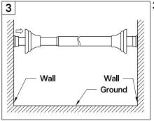
3. Holding the larger sized rod, rotate the smaller rod until it is locked into position securely.
