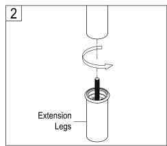
Thread the extension legs onto the original legs by turning clockwise.
