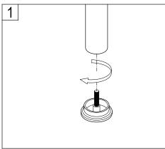
Remove the floor flanges from the original legs by turning counter-clockwise.
