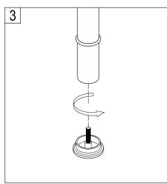
Thread the floor flanges onto the extension legs.
