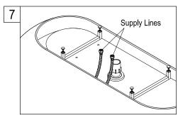
7. Install faucet on tub as per manufacturer's instructions and attach flexible supply lines to the faucet, these lines should be long enough to extend 4" to 8" beyond the bottom of the tub.
