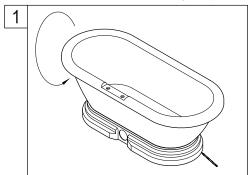
1. Position the tub at the desired location, with a pencil mark the perimeter of the base, also mark the location of where the tub drain will be situated, and place the tub upside down on a blanket or piece of cardboard.
