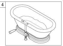
4. Close the drain and fill the tub with 2" to 5" with water, while inspecting the connection from below the floor, drain the tub and check for leaks. Apply caulking around the perimeter as needed, clean excess caulking.
