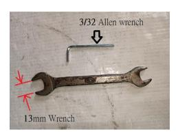
Step 1: Use allen wrench (3/32" size) to loosen the set screw and pull out the spout
