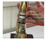
**Step 7:** Tighten up the set screw with allen wrench
