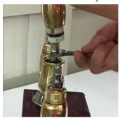
Step 6: Adjust and make sure the upper C-clip's small hole is to align with set screw hole of the body
