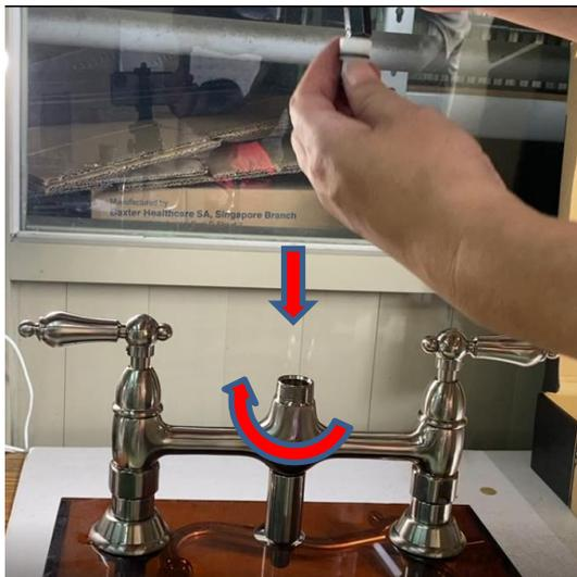
Insert new Diverter into the well and lock in place by threading it in place (about 4-5 turns) using 12mm Hexagonal Allen Wrench.
