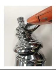
Carefully insert a thin screwdriver into the gap between the top finial and the handle.
