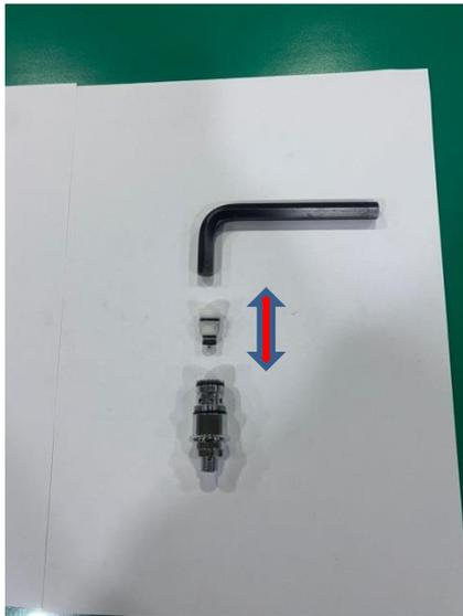
Use a 12 mm Hex Allen wrench to loosen the diverter from the adapter by turning counter-clockwise. Clean all impurity or debris inside the adapter body and then install a new diverter onto the adapter by turning clockwise.
